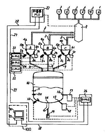
ABSTRACT: PROBLEM TO BE SOLVED: To provide an automatic raw material compounding device for automatically and totally controlling respective processes of raw material compounding, raw material metering and the like.
